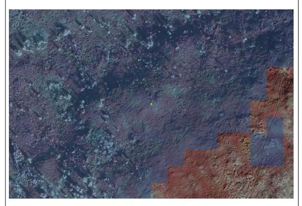
**Fig. 7** Commission error for bushy non-tree vegetation in Northern Finland. Also the area where no tree tops are present was erroneously classified as tree cover. (7774815, 533900)
