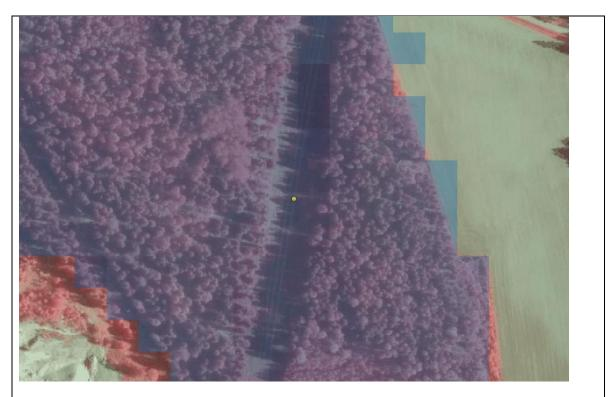
**Fig. 10** Commission error on power lines in forest area. Here no visible tree crowns underneath the power line. In surroundings like this, ground under the power line grows seedlings or young forest due to natural regeneration, and is maintained by clearing as the trees grow too high. Thus, correct classification is challenging (6747256, 408378).
